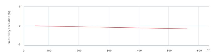
ISO 9001 certified calibration at  $+20^{\circ}$ C with dead weight tester (3, 6, 8, 10, 12, 20, 30, 50 bar). Sensitivity and linearity are determined according to DIN16086
