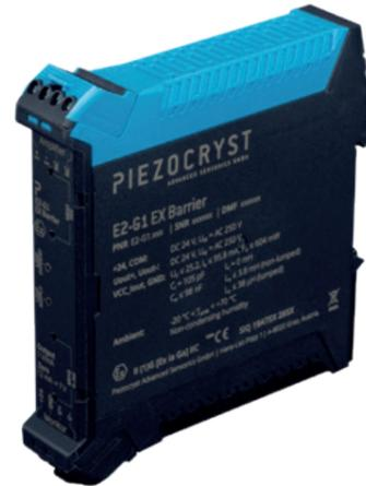
The Piezocryst E2-G1 EX barrier and galvanic separation unit is designed to complete the measurement chain of CP- or G-series transducers with the E2-Ax differential charge amplifiers. This unit enables the CP-series and G-series sensors, including E2Ax charge amplifier, to be installed in hazardous areas up to Ex zone 0. Two LEDs show whether the correct power supply and current loop to the charge amplifier are present, indicating the health of the electronic installation.
