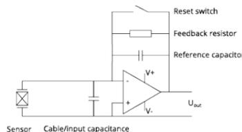
Working principle of an amplifier with reset and feedback resistor
